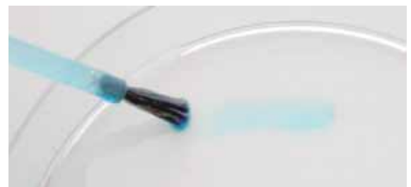
fig. 42: treated surface (72 mN/m)
