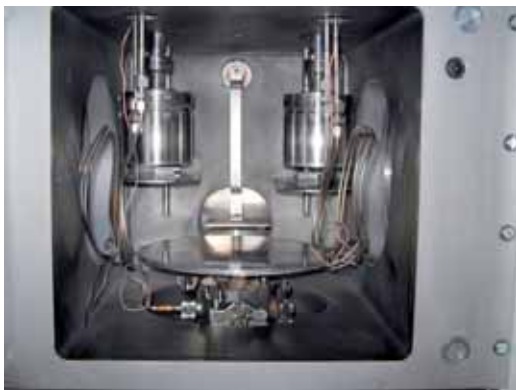
fig. 79: view into the vacuum chamber of a sputtering coating system. You can see two sources of sputtering of cylindrical geometry here. During the coating process are the substrates under the sources on (swivelling) the plate (top down arrangement). For the in-situ control of the coating rate and the layer thickness are two independently working measuring systems installed.
