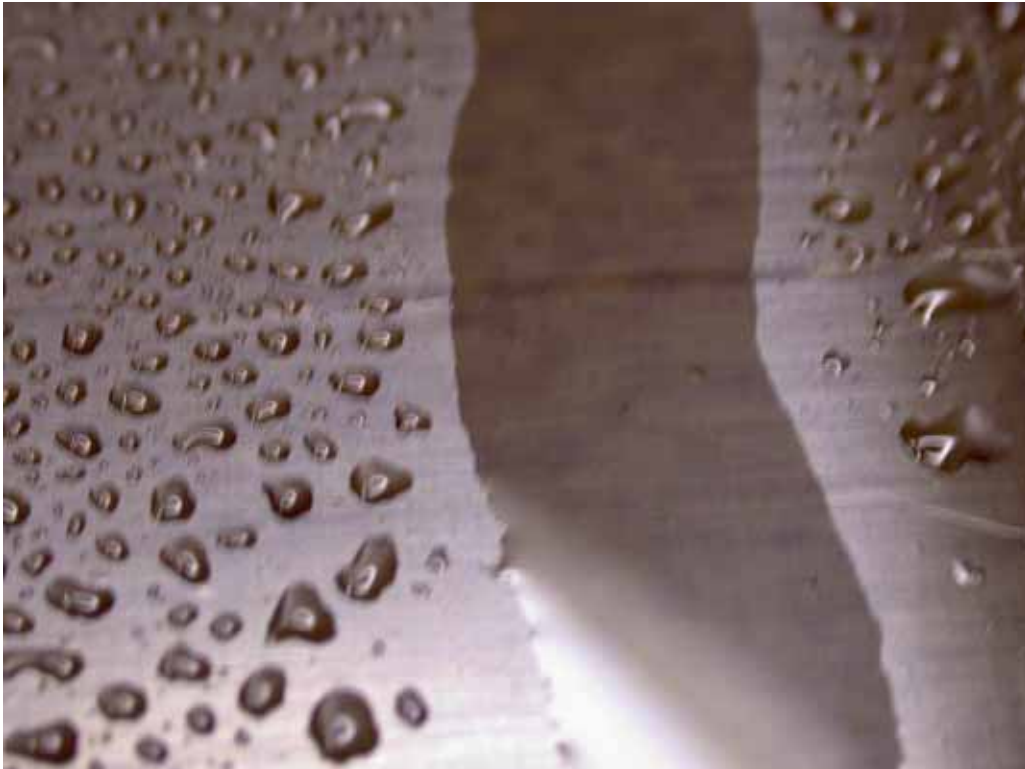
fig. 165: difference: plastics with and without plasma treatment
