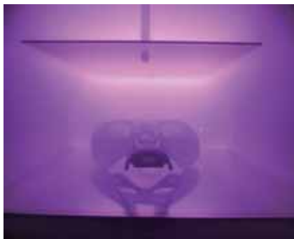
fig. 17: oxygen plasma, high pressure
