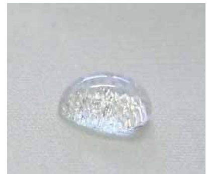
fig. 61: treated cotton (isopropanol)
