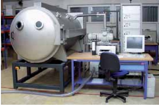
fig. 104: plasma system TETRA-2400-LF-PC designed for the production
