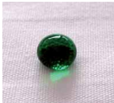
fig. 60: treated cotton (water) hydrophobic
