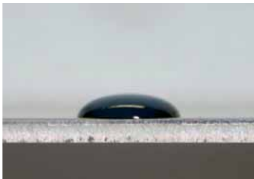
fig. 57: Metal surface untreated
