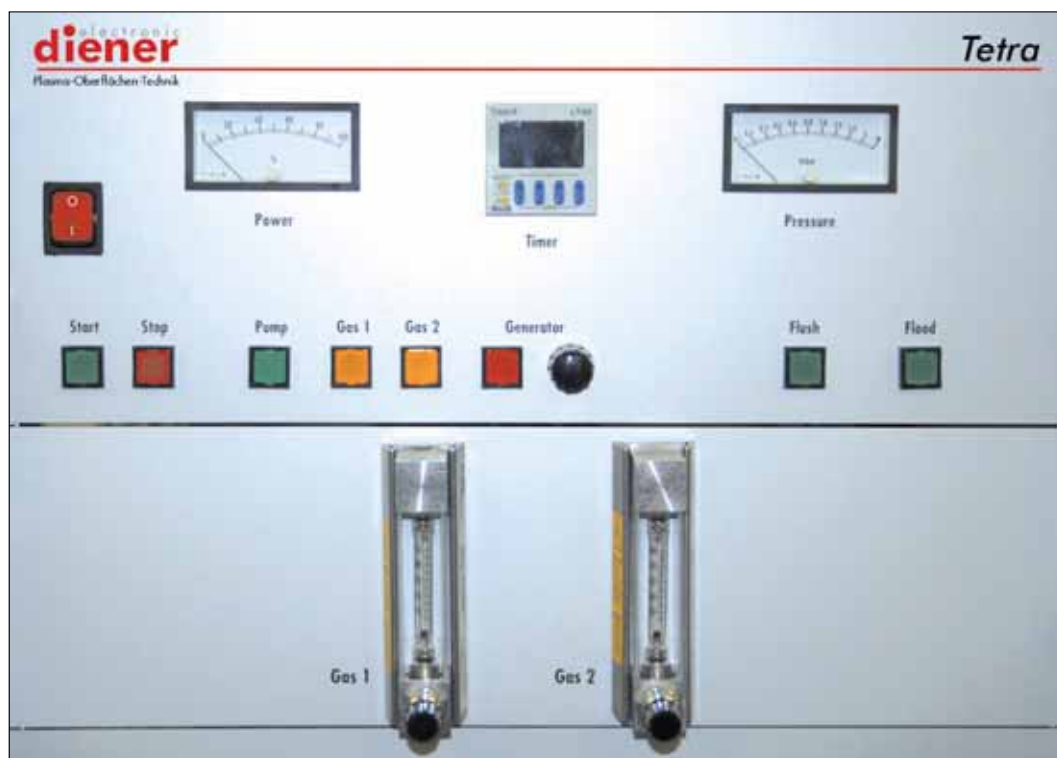
fig. 112: controls of a TETRA Plasma system
