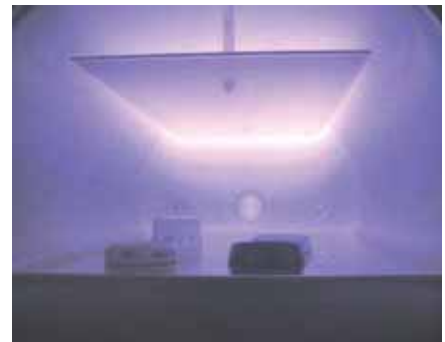
fig. 18 : oxygen plasma, low pressure
